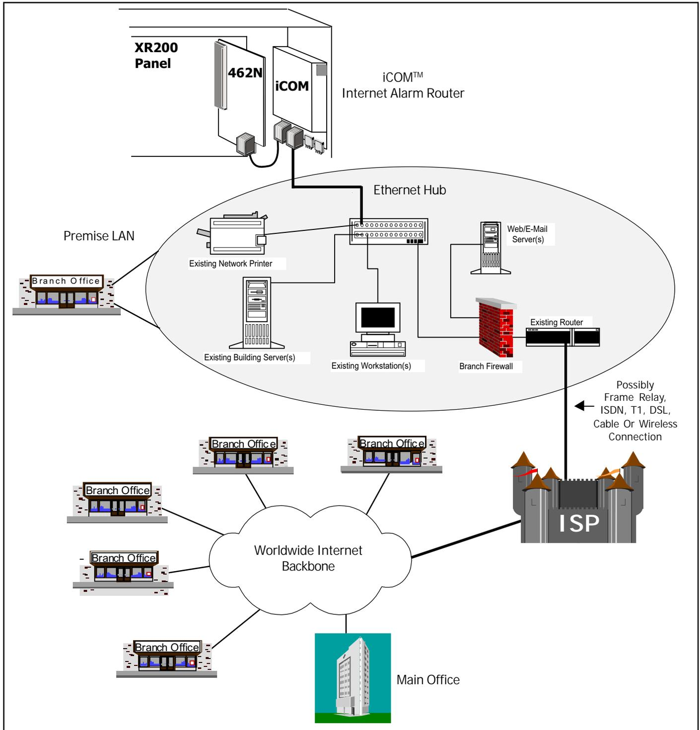
Figure 2: Typical corporate network with XR200 panel
