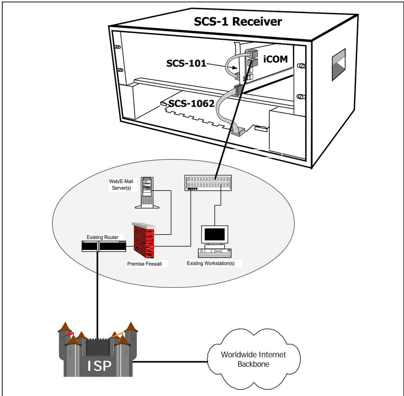
Figure 3: Typical Internet Monitoring configuration for central station
